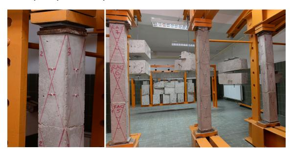
FIGURE 3.25: Prisms positioned in the frame
