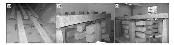
FIGURE 2.23: Test setup of long-term experiment: (a) Shrinkage beam; (b) Simply supported beam; and (c) Continuous beam, (Liu et al., 2008)
