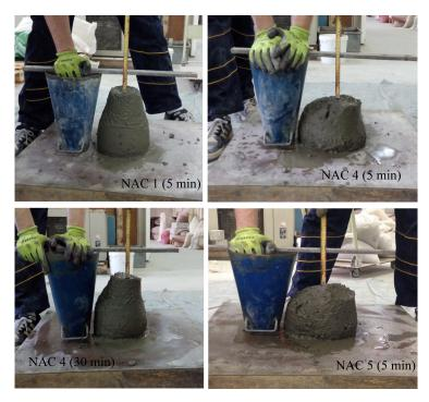
FIGURE 4.2: Slump measurements – NAC
