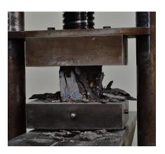
FIGURE 3.18: Compressive strength testing
