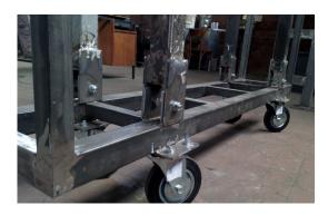
FIGURE 3.32: Steel cart aligned with steel 'hands'
