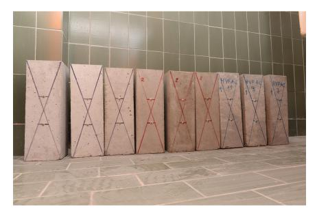
FIGURE 3.23: Prisms for measuring shrinkage
