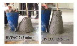
FIGURE 4.4: Slump measurements – HVFAC
