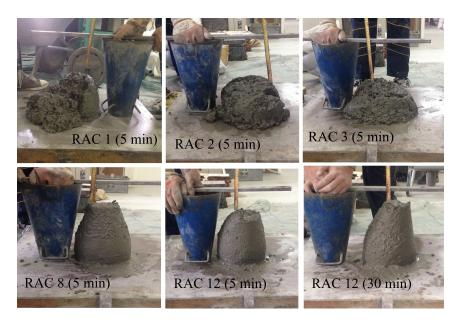
FIGURE 4.3: Slump measurements – RAC
