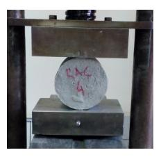
FIGURE 3.19: Splitting tensile strength testing
