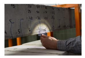
FIGURE 3.42: Measuring crack widths with a crack gauge
