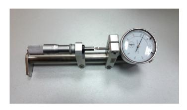
FIGURE 3.36: Calibration of dial indicator
