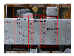
FIGURE 4.39: Close view of middle cross-sections of beam RAC7
