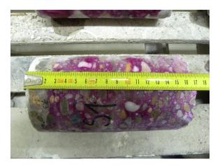
FIGURE 3.4: Column core carbonation
