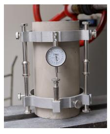
FIGURE 3.21: Modulus of elasticity testing
