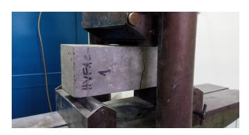
FIGURE 3.20: Flexural tensile strength testing
