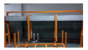
FIGURE 3.30: Steel 'hands' on beams
