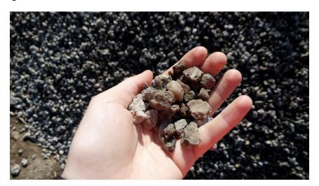
FIGURE 2.14: Recycled concrete aggregate particles
