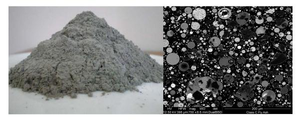
FIGURE 2.22: Fly ash sample (left) and scanning electron microscopy (SEM) image (right)
