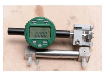
FIGURE 3.22: Mechanical strain gauge
