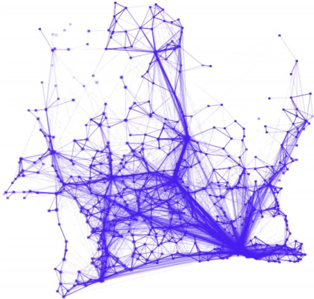
Figure 3.3: Trajectory aggregation model based on OPTICS “route similarity” clustering
