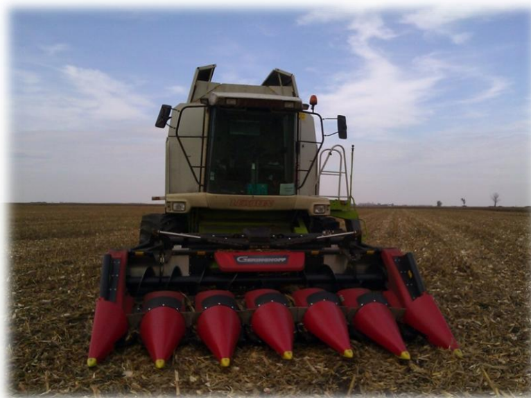
Slika 6.14 Kukuruzni adapter GERONGHOFF MS HORIZON 670
