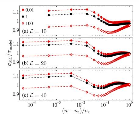
Figure 3.10: The conductivity ratio between the MC simulation results  $\sigma_{\rm MC}$  and the values obtained from the model  $\sigma_{\rm model}$  given by Eq. (3.11) for different system sizes (a)  $\mathcal{L} = 10$ , (b) 20, and (c) 40 and for three conductance ratio values  $G_{\rm j}/G_{\rm s} = 0.01$ , 1, and 100. The error bars are smaller than the size of the points.
