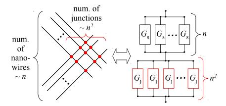
Figure 3.5: Schematic illustration of simplified model of random NW network where the total number of junction is proportional to the square of normalized NW density  $n^2$  (left panel). The equivalent conductance of the simplified network presented as serial conductance n NWs in parallel and  $n^2$  junctions in parallel (right panel).
