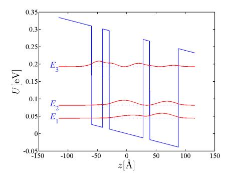
Figure 5.1: The conduction-band diagram of the active region of GaAs/Al<sub>0.33</sub>Ga<sub>0.67</sub>As QCL described in Ref. [64], in an electric field of 44 kVcm<sup>-1</sup>. The subband positions at zero magnetic fields, together with the corresponding wave functions squared, are also displayed.
