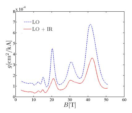
Figure 5.8: The optical gain (per unit injection current) as a function of the applied magnetic field in the range B = 3-60 T at temperature T = 300 K.
