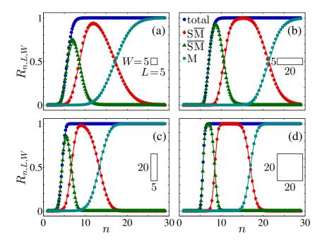
Figure 4.8: The percolation probability functions of two symmetric (a) and (d) and two asymmetric systems (b) and (c). Different percolation characteristics are shown: for overall CNT percolation  $R_{n,L,W}$  and for three operation regimes  $R_{n,L,W}^{\overline{SM}}$ ,  $R_{n,L,W}^{\overline{SM}}$ , and  $R_{n,L,W}^{\overline{M}}$ . The points are the MC simulation results and the solid lines are obtained using Eqs. (2.28) and (4.3)-(4.5).
