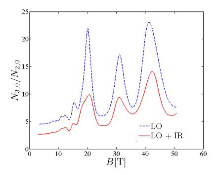
Figure 5.7: The ratio of the total electron areal densities due to the electron LOphonon and interface roughness scattering, in the ground laser levels of the third and the second subband, as a function of the magnetic field and at temperature T = 300 K.
