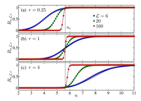
Figure 2.9: The percolation probability functions for different aspect ratios (a) r = 0.25, (b) 1, and (c) 4 and for three normalized system size values  $\mathcal{L} = 6$ , 20, and 160. The points are obtained from the MC simulations and calculated using Eq. 2.2. The solid lines denote values obtained from our analytic model for the percolation probability functions given by Eq. (2.28). The vertical dashed lines denote the percolation threshold value  $n_c$ .
