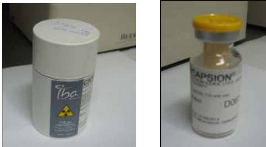
Figure 25. Lead container and vial for the capsule
