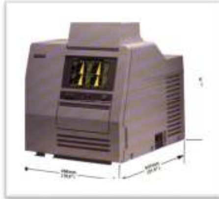
Figure 22. TLD Reader Thermo Harshaw 6600
