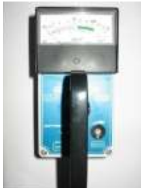
Figure 19. Survey meter "mini-rad" series 1000
