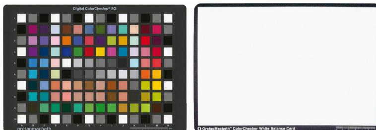
Slika 5.10. Test karte korišćene u istraživanju (a) Digital Color Checker SG test karta, (b) Color Checker White Balance test karta (X-Rite, 2009)
