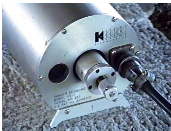
Sl. 7.7 Seizmometar SS-1 Ranger
