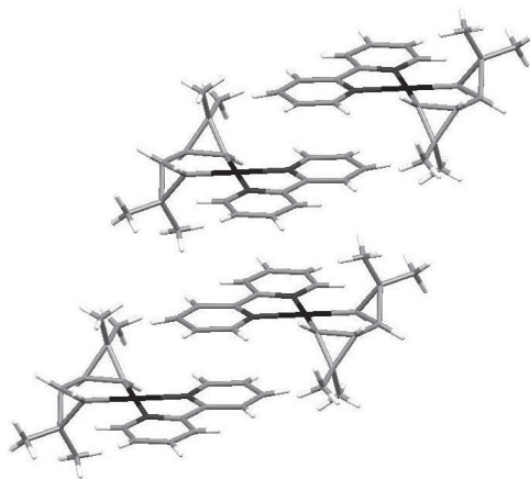
Figure 3.14. The perspective view of crystal fragment of PNIHEP 409 ((2,2'-bipyridyl)-5-nickela-3,3,7,7-tetramethyl- trans -tricyclo (4.1.0.0 2,4 )heptane), as an example of stacking chains with repeating the same overlap; in this case the other ligand is voluminous.
