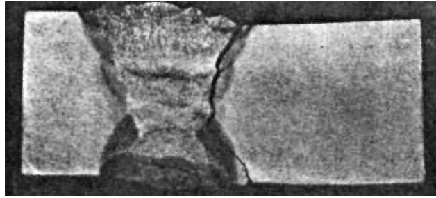
Figure 1-2. Macro-cracks in HAZ in NIOVAL 47 steel welded joint, [2]
