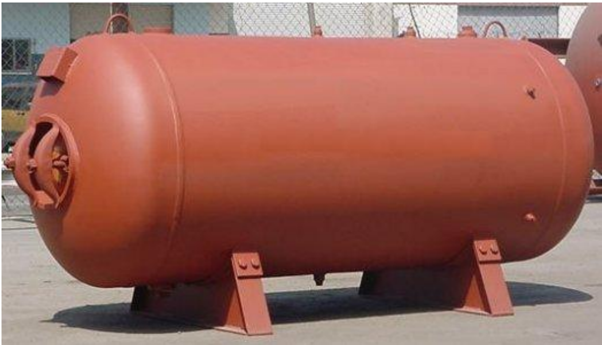
Figure 2-1. Horizontal cylindrical pressure vessel in steel
