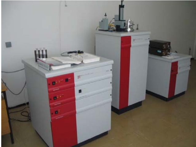
Slika 4.14. Quantum Design MPMS XL-5 SQUID magnetometar, INN Vinča
