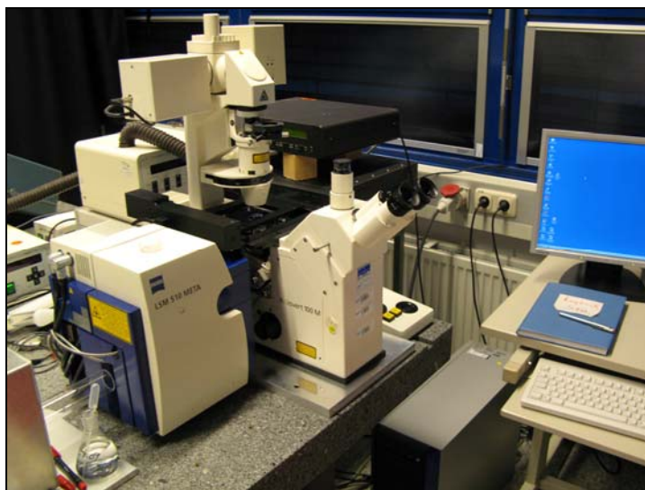
Slika 17. Konfokal laser skening mikroskop, model LSM-510-META (Germany)
