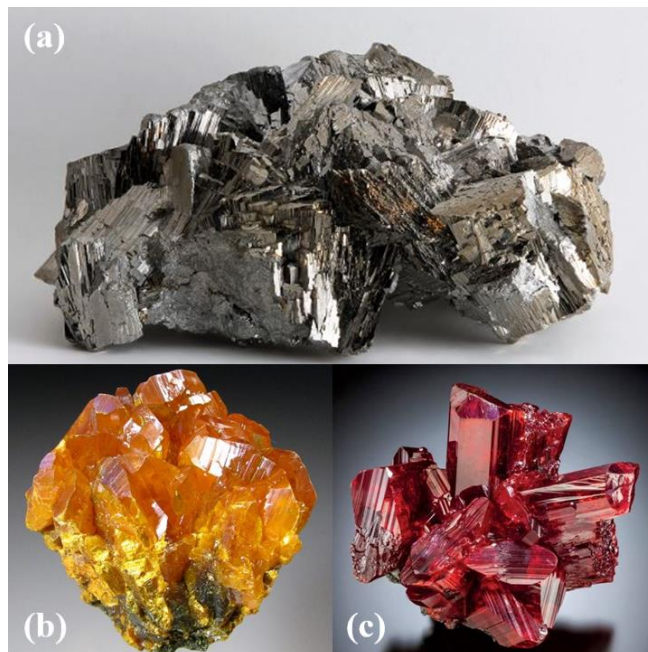
Slika 2. Minerali arsena: (a) arsenopirit ( \text{FeAsS} ), (b) orpiment ( \text{As}_2\text{S}_3 ) i (c) realgar ( \text{AsS} ).
