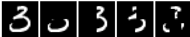
Figure 6.1: Example of digit 3 in our validation set; From left to right: unmodified – original version, horizontally cut image – top half removed, vertically cut image – left half removed, diagonally cut image – first and third quadrants removed, "triple cut" image – three squares removed as described before.
