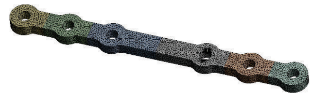
Figure 8 Plate C mesh with initial cracks
