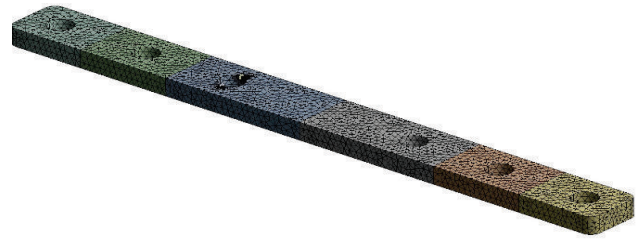
Figure 6 Plate A mesh with initial cracks
