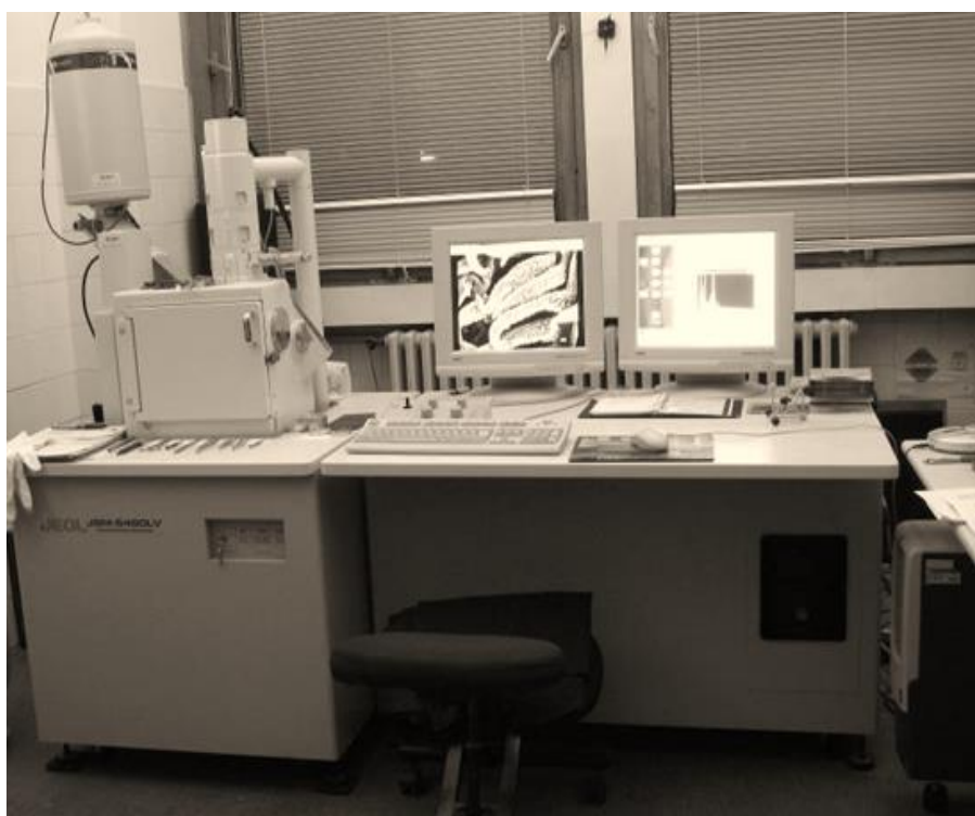
Fig. 3.10 Scanning Electron Microscope SEM JEOL JSM-6460LV, Novi Sad
