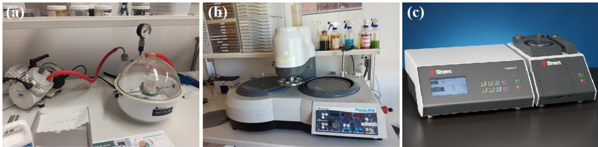
Fig. 3.8 (a) Buehler Cast N' Vac 1000 vacuum chamber; (b) Buehler Phoenix 4000 sample preparation systems; (c) Struers LectroPol 5 electropolisher
