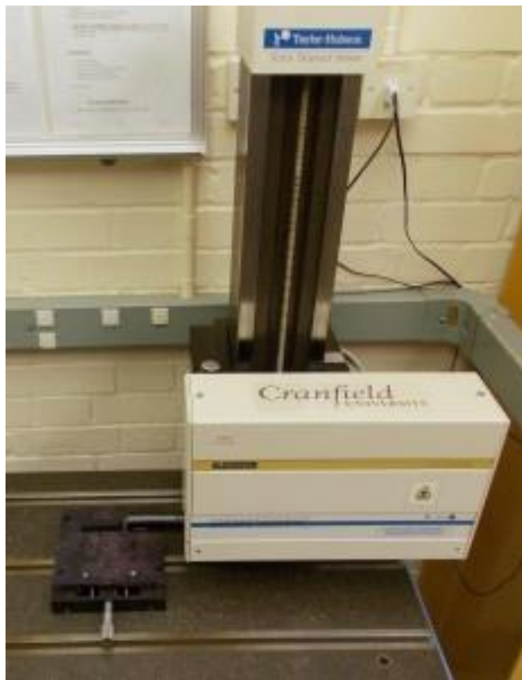
Fig. 3.6 Contact mode surface profilometer (Taylor Hobson Form Talysurf Series 2)
