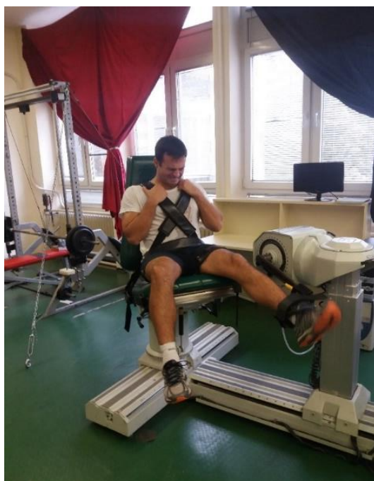
Picture 3. Testing set-up for knee extension and knee flexion test
