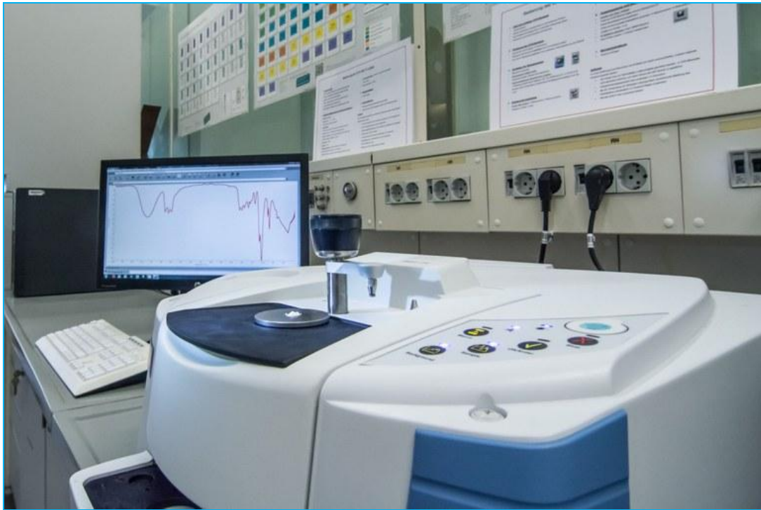
Figure 32. Nicolet IS10 FTIR spectrometer.
