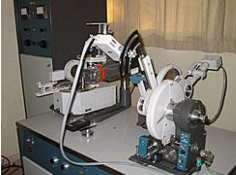
Figure 29. Philips PW1050 diffractometer PW1050.
