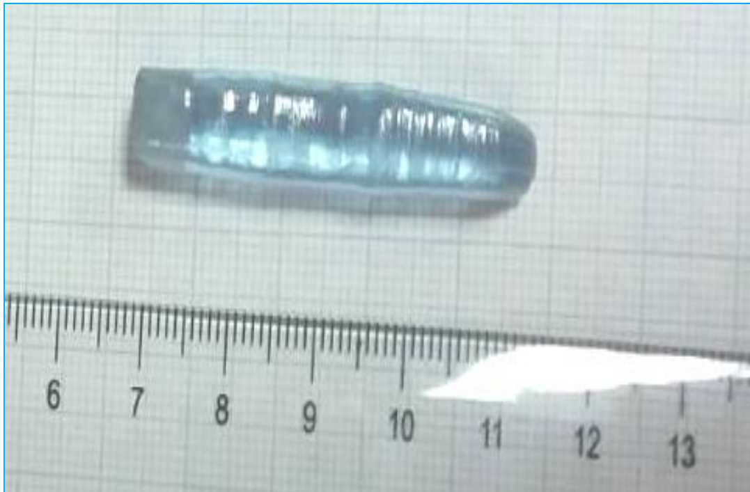
Figure 35. Photographs of \text{CaWO}_4:\text{Nd}^{3+} single crystal [23].
