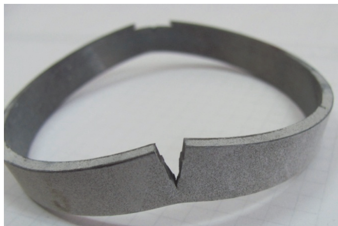
Figure 7.2. One of the specimens with prominent crack growth
