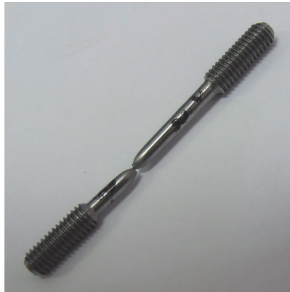
Figure 7.28. A broken RT specimen
