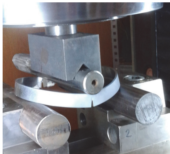
Figure 6.32. Side of the specimen for Aramis measurement, with applied contrast spray (specimen already deformed)
