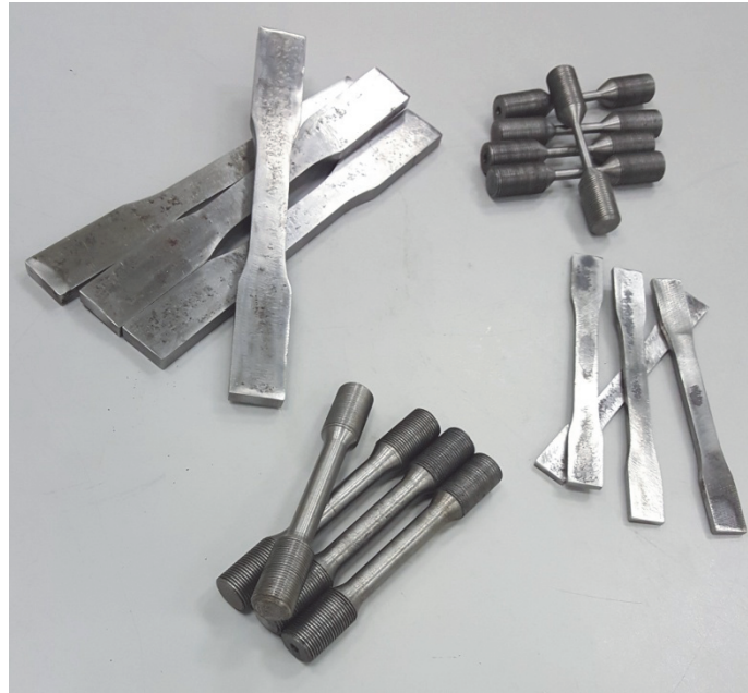
Figure 6.10. Geometries of tensile specimens [96]
