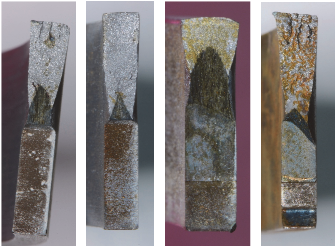
Figure 7.5. Fracture surfaces of ring-shaped specimens
