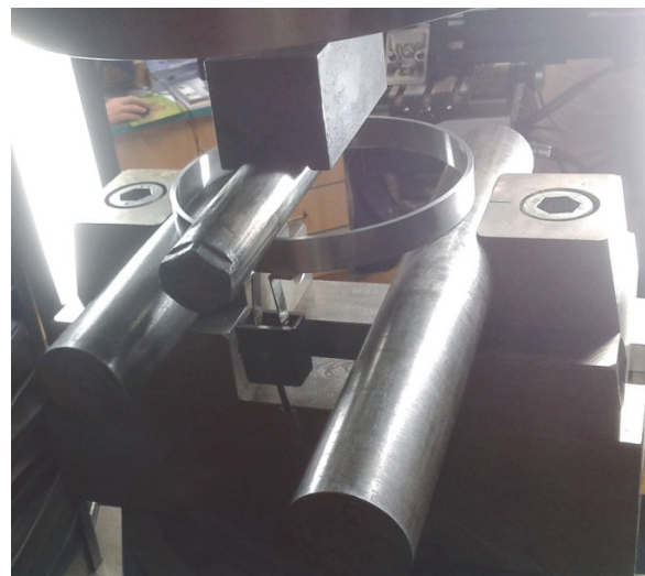
Figure 6.34. Side of the specimen with COD gauge
