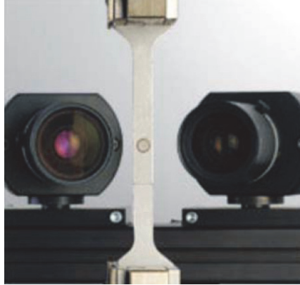
Figure 6.22. Cameras of Aramis system with the tested sample at the centre. [97]
