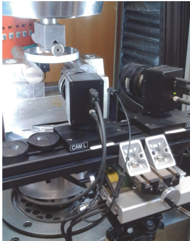
Figure 6.31. Testing equipment: tensile testing machine and stereometric measurement system
