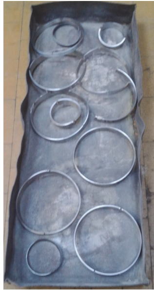
Figure 7.3. Specimens prepared for heating in the furnace
