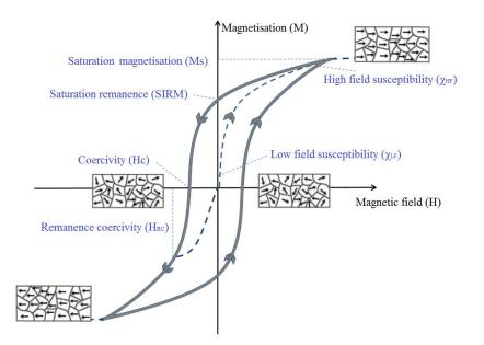
Figure 2.3 Ferromagnetic material magnetic hysteresis (M-H) loop and magnetic properties most usually applied in the studies of magnetic measurements; The susceptibility (low and high field – shown by the M-H curve slope); initial magnetisation (dashed line in upper right quadrant on the graph) and the samples' magnetic remanence at remanence coercivity (lower left quadrant) (adopted and modify from Hofman et al, 2017).
