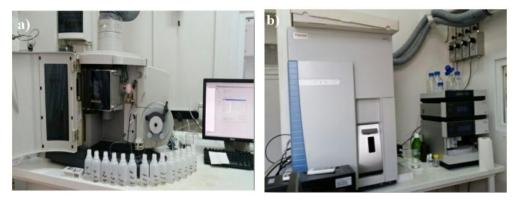
Figure 3.11 a) Inductively coupled plasma-optical emission spectrometry (ICP-OES); and b) inductively coupled plasma-mass spectrometry (ICP-MS).
