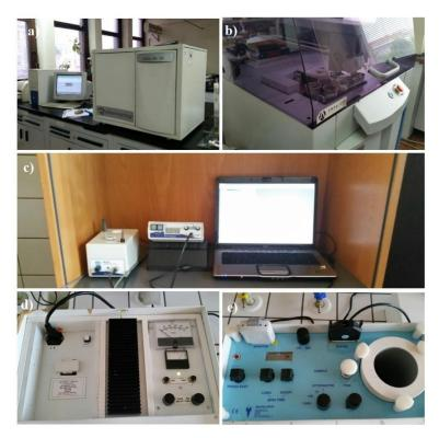
Figure 3.12 a) Elemental C, N, H, S Analyser; b) WD-XRF; c) Magnetic susceptibility-meter; c) magnetiser; d) magnetometer (Molspin Minispin magnetometer).
