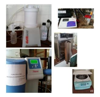
Figure 8.1.1 a) distillation for preparing acid (p.a.) for the samples digestion; b) distillation for preparing ultra-pure water used for the samples preparation; c) pH-meter d) dryer; e) centrifuge.
