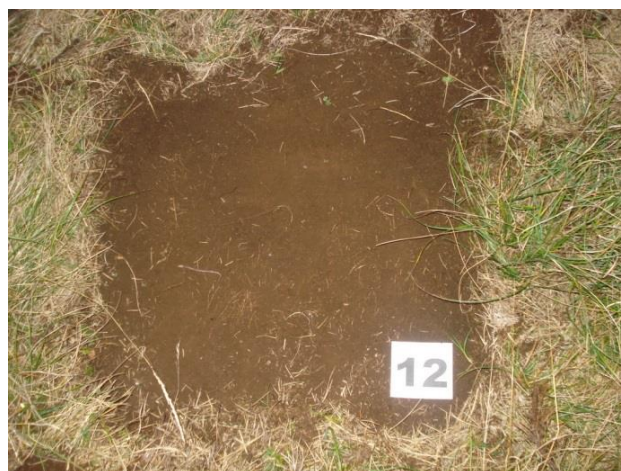
Figure 7 Soil sampling (preparation for soil collection - removal of surface vegetation, stones and fauna on sampling site 12)
