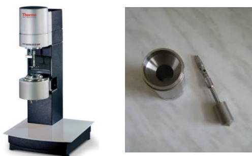
Figure 31. RheoStress 600, Haake and accessories used in the rheological analysis of confectionery fat filling
