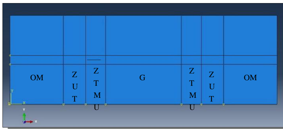
Slika 5.20 Zone u FSW spoju-3D model
