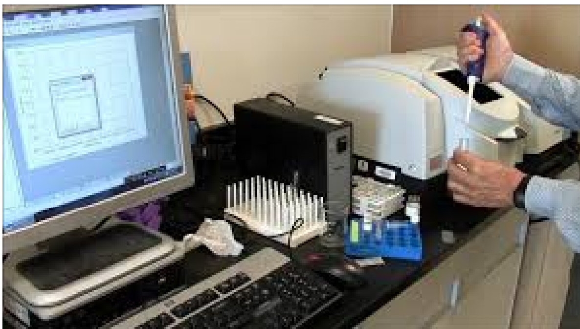
Figure 12. Spectrophotometer Evolution UV-VIS 300.
