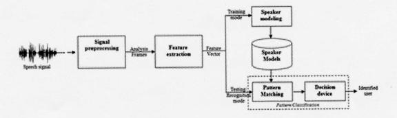
Figure 1. General speaker recognition system architecture.6
