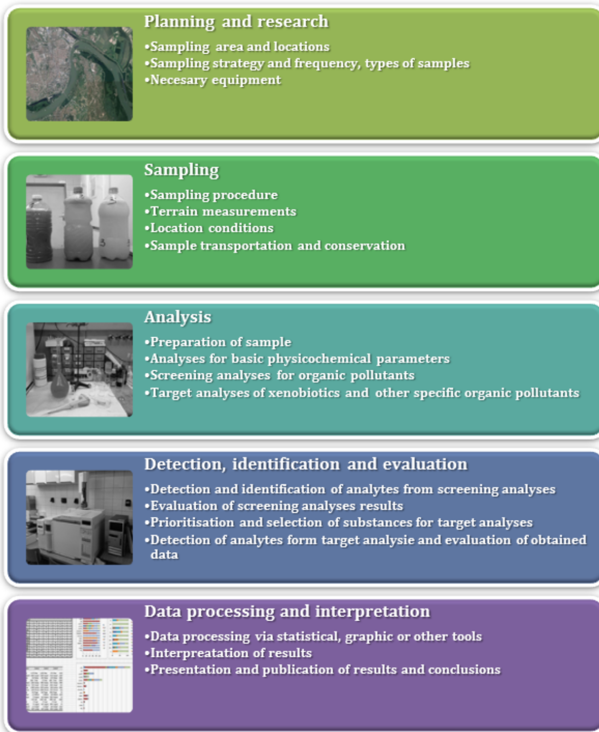
Figure 5.10 Modules of emerging xenobiotics detection in urban wastewater
