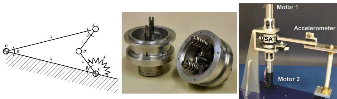
Figure 1.14. Functional scheme of VSA-II (4-bar transmission mechanism). Link OA is driven by a motor at O . The torque spring k is linear, while stiffness seen at O attains non-linearity through geometry (left); VSA-II prototype (middle); Test-bed for evaluation of VSA-II integration into a robotic joint (right).
