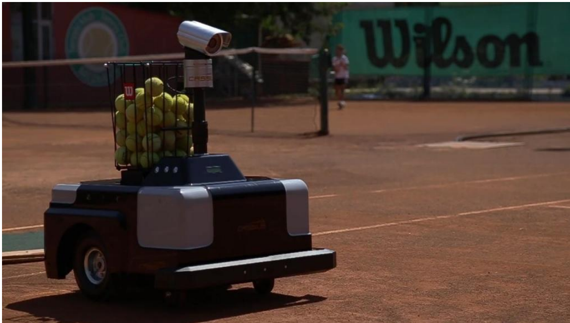
Figure 2.13. Robot Cassius – one of the first robots that assists tennis players. It has been developed by Morena Engineering and is capable of rolling clay tennis courts between games. The dynamic balance of the robot needs to be thoroughly analyzed and its mobile base shaped to cover every possible, added, highly inertial interaction task, such as throwing tennis balls.
