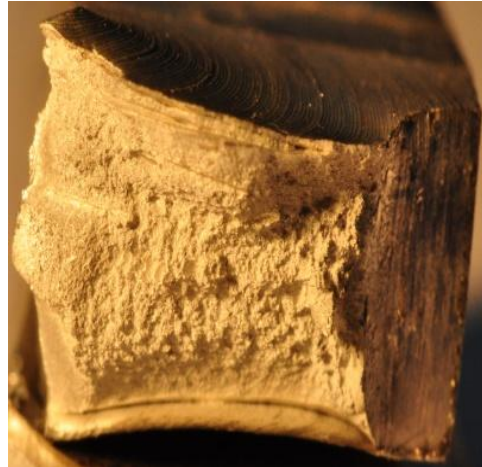
Fig.4-12d 2 . Macrophoto. fracture (800rpm,75mm/min)
