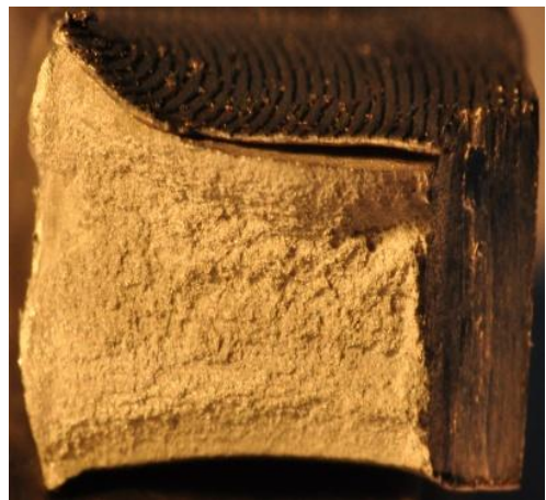
Fig.4-12o 2 . Macrophoto. fracture (500rpm,150mm/min)
