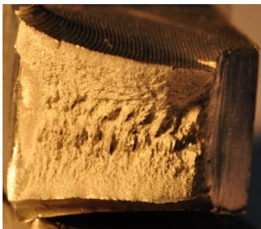
Fig.4-12f 1 . Macrophoto. fracture (600rpm,100mm/min)
