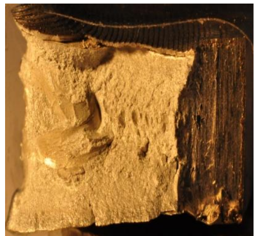
Fig.4-12i 2 . Macrophoto. fracture (500rpm,125mm/min)
