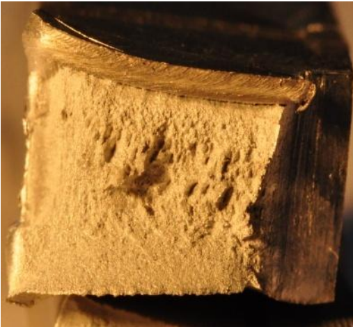
Fig.4-12e 1 . Macrophoto. fracture (500rpm,100mm/min)
