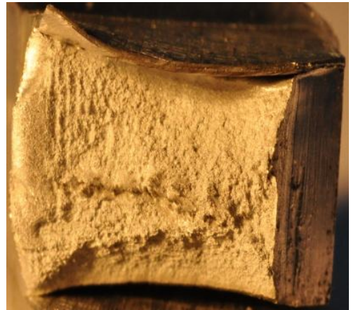
Fig.4-12h 2 . Macrophoto. fracture (800rpm,100mm/min)
