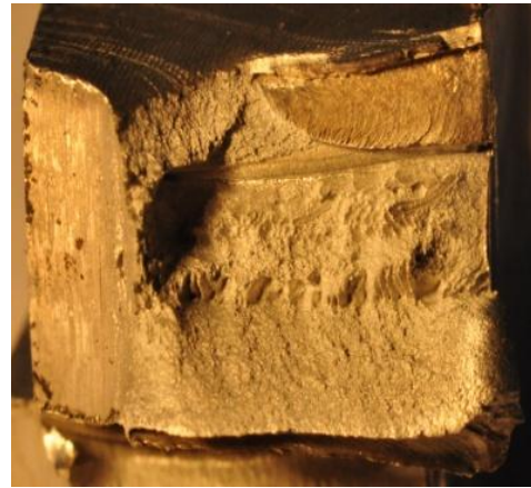
Fig.4-12b 2 . Macrophoto. fracture (600rpm,75mm/min)
