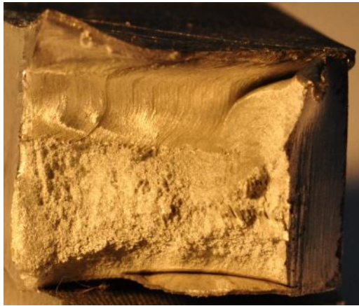
Fig.4-12k 1 . Macrophoto. fracture (700rpm,125mm/min)
