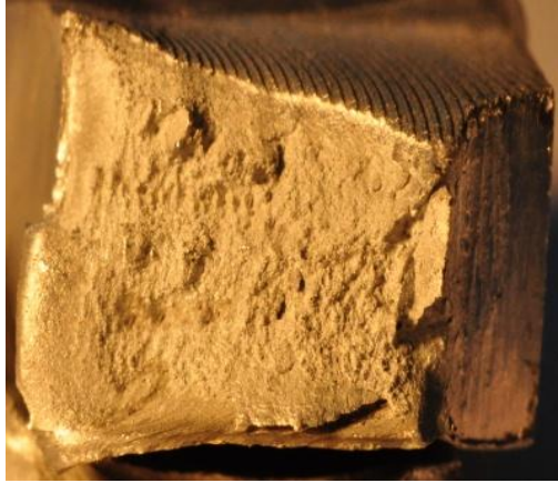
Fig.4-12n 1 . Macrophoto. fracture (600rpm,150mm/min)
