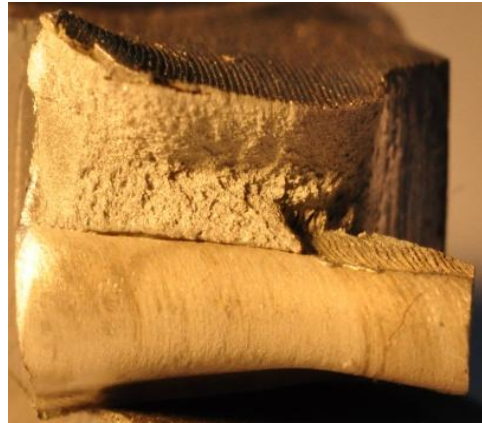
Fig.4-12l 2 . Macrophoto. fracture (800rpm,125mm/min)
