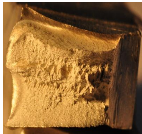
Fig.4-12f 2 . Macrophoto. fracture (600rpm,100mm/min)
