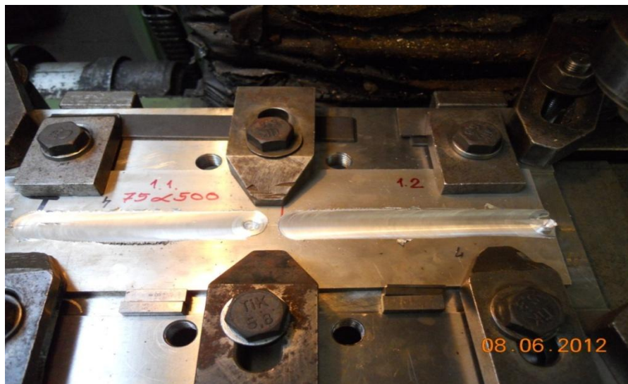
Figure 3-5. Clamps of work piece to machine FSW.
