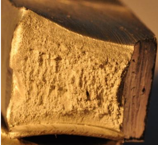
Fig.4-12d 1 . Macrophoto. fracture (800rpm,75mm/min)
