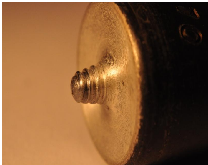
Figure 3-3. Tool Probe (Pin) with Tread Right Hand.
