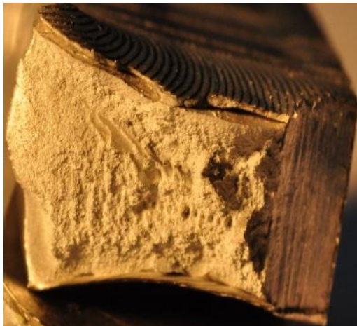
Fig.4-12i 1 . Macrophoto. fracture (500rpm,125mm/min)
