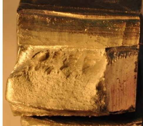
Fig.4-12a 2 . Macrophoto. fracture (500rpm,75mm/min)
