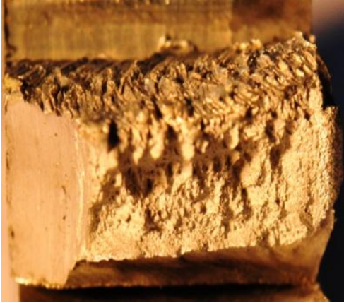
Fig.4-12a 1 . Macrophoto. fracture (500rpm,75mm/min)
