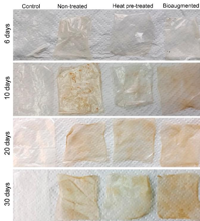
Figure 5. PVA/TPA film samples after compost burial at different time points.
