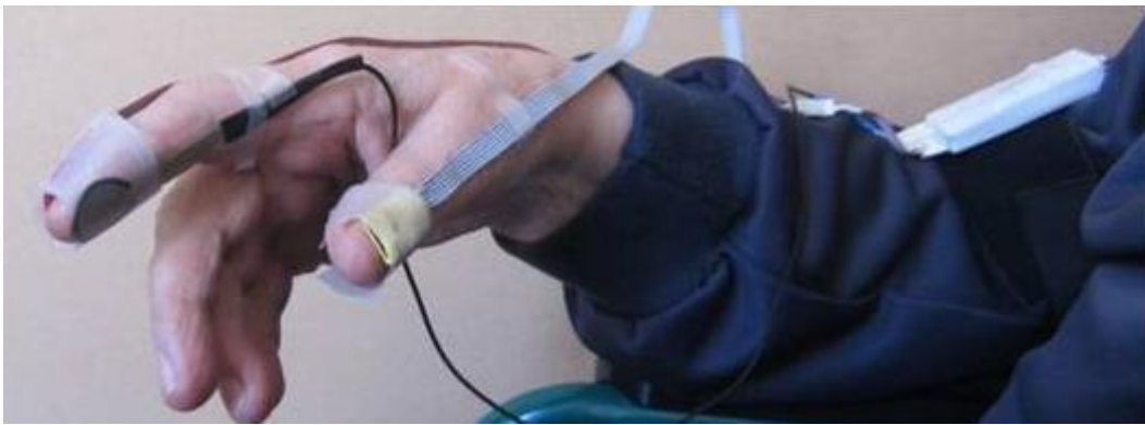
Figure 7 Wearable system used to record kinematic data (Image adapted from [110])
