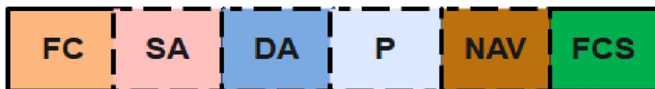
Figure 3.3: Frame structure of Tx-Beacon. DA and P represent destination address and priority value, respectively.
