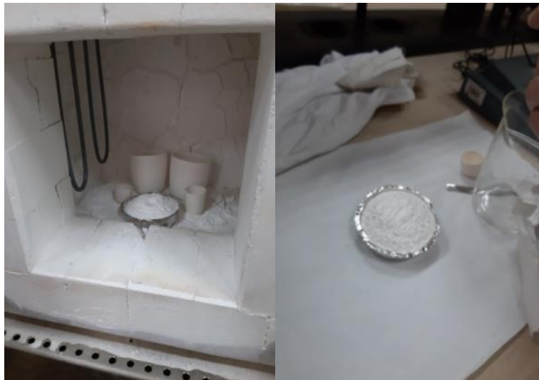
Figure 21. Furnace for thermal treatment (calcination) of HAp and the obtained \alpha -TCP powder.
