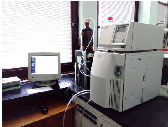
Slika 5. HPLC: 1500 Series HPLC, Waters sa UV detektorom 2487 Dual \lambda Absorbance Detector, Waters.
