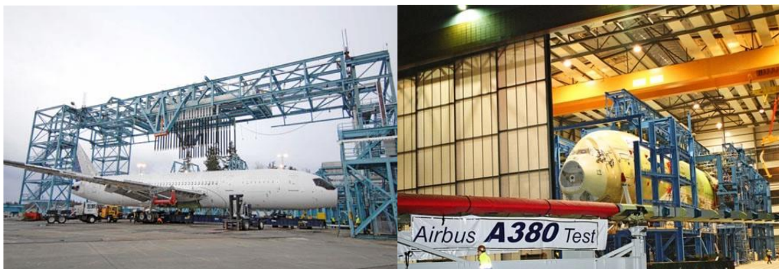
Sl.70. Zamorni test (Full scale test) B787 i A380 [85, 86]
