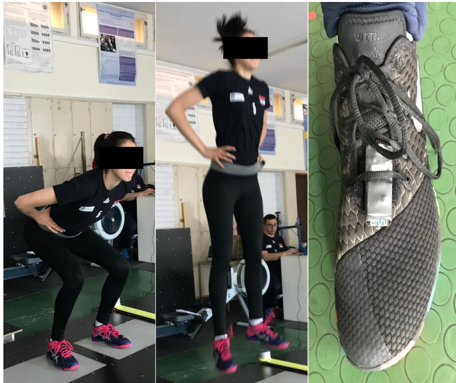
Figure 10.3: Squat jump - starting (left), take-off/landing position (middle), and kinematic sensor device placement (right)
