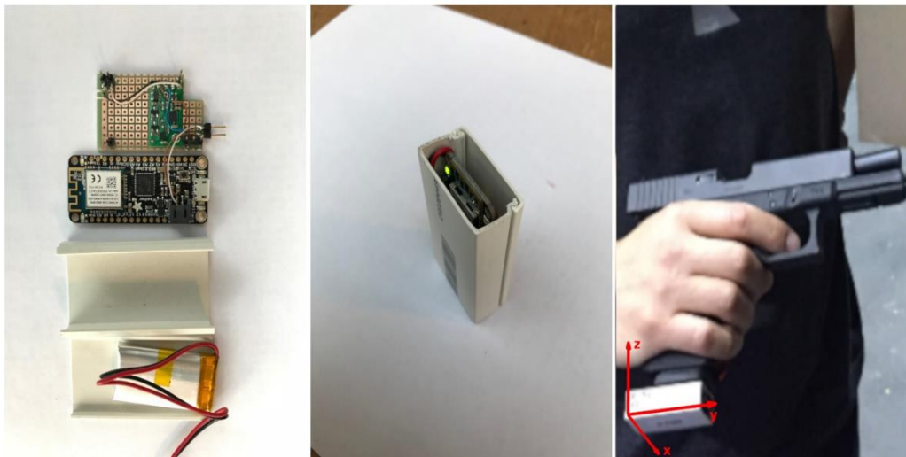
Figure 8.1: Left – sensor device components 6 DoF sensor, microcontroller with Wi-Fi communication module, battery, and encasement; Center – fully assembled sensor device; Right – sensor device mounted onto the bottom of the pistol grip
