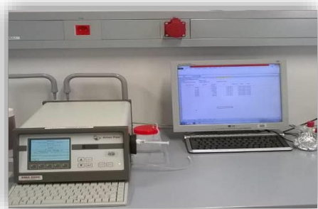
Slika 3.1. Automatski denzimetar a) Anton Paar DMA 5000 i b) Rudolph Research Analytical DDM 2911 .
