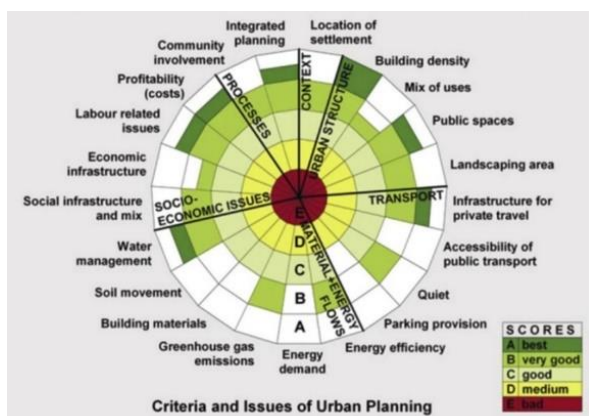
Fig. 3. Evaluation compass for criteria used in the Ecocity assessment tool. Adapted from Gaffron et al. (2008).
