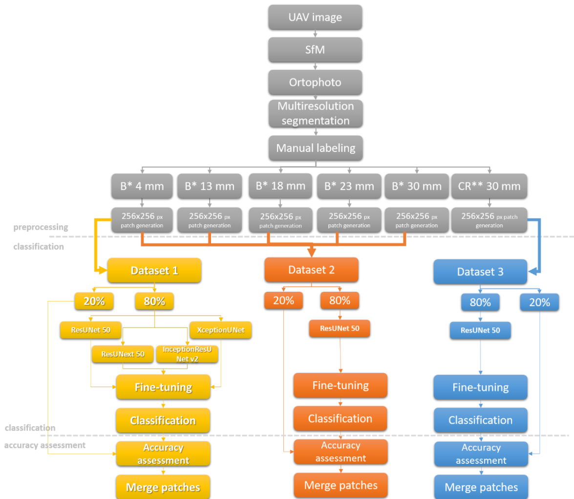
Figure 36. Workflow used in this study where “B*” and “CR**” correspond with the Balkana and Crna Rijeka dataset respectively. UAV = Unmanned Aerial Vehicles; SfM = Structure from Motion
