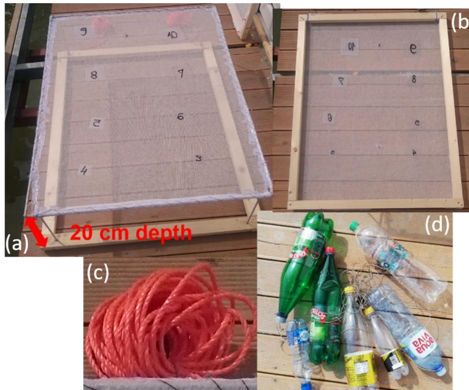
Figure 35. Targets used in the study area located in Lake Balkana (a) frame with metal construction for the underwater survey, (b) frame for the on the water surface survey, (c) nylon rope, (d) plastic bottles.
