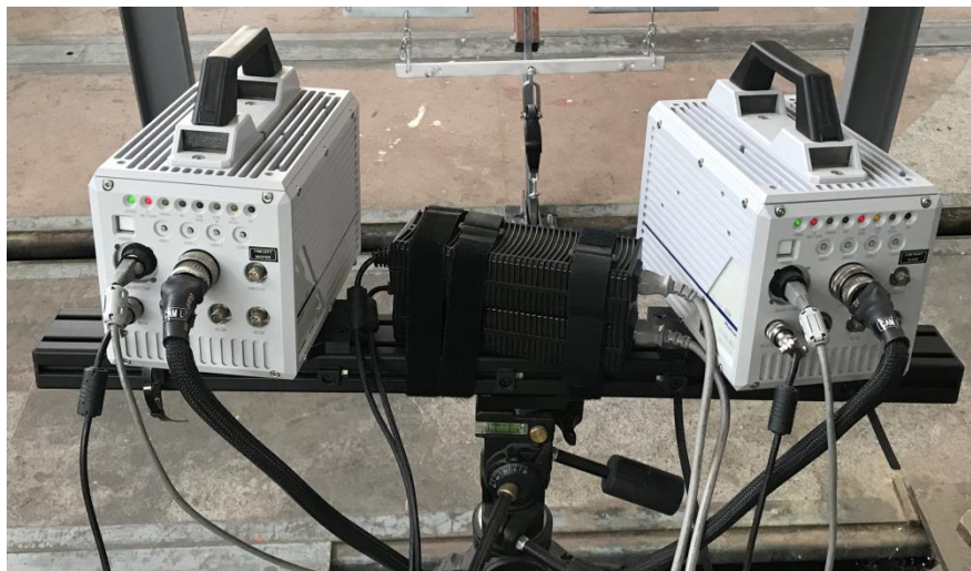
Figure (5.66) 3D DIC system used
