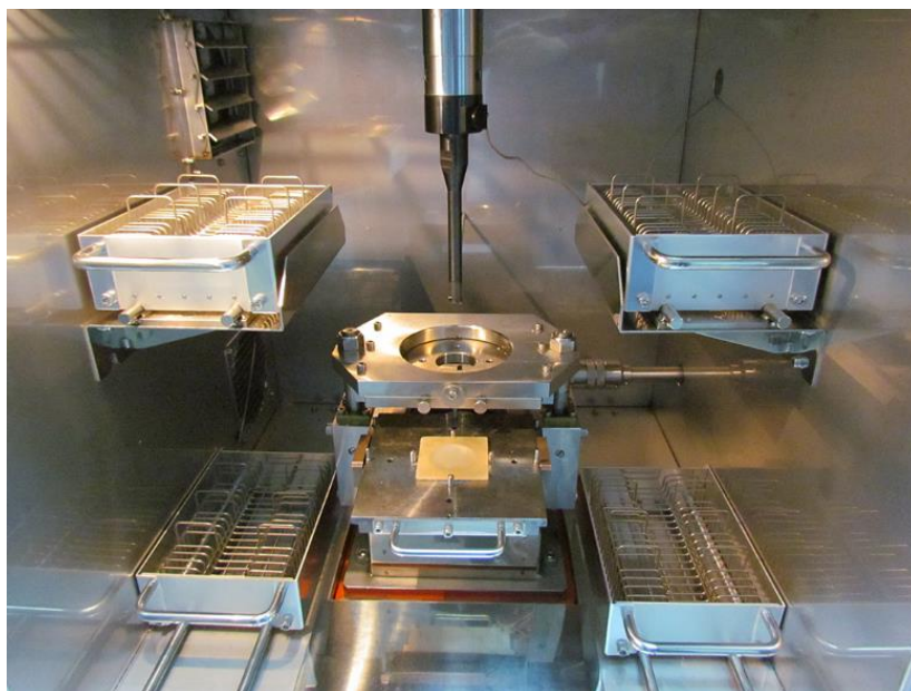
Figure 32. “Specimen for high-speed impact testing in the testing machine after impact” [87].
