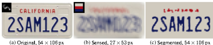
Fig. 2 Segmentation of a heavily blurred licence plate. Original image (a) is blurred with PSF shown in the top left corner of (a), and then subsampled 2\times to create the sensed image (b). Segmentation of (b) by the proposed method (SRCS-HTVF; see Sec. 3) using a three-component end-member matrix [shown as colored stripes in the top left corner of (b)] at 2\times increased resolution provides the segmentation (c) (shown as a composite of the three components). The larger blue characters are well segmented, whereas the smaller red characters demonstrate limits of the method's performance.
