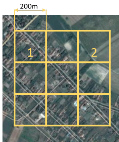
Figure 7.9: A high resolution satellite image, with a superimposed 200 meter resolution grid, illustrating the pixel size of presented satellite image. Pixel #1 is a fairly homogenous pixel, almost completely covered by urban area, whereas pixel #2 is mixed pixel, partially covered by vegetation and soil.
