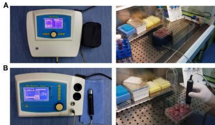
Fig. 2 Application of physical therapy modalities on hAT-MSC culture in vitro. a Magnet therapy device (EkoMedico, Electronic Design, Belgrade, Serbia) and application of magnet therapy (50 Hz, 3 mT, 30 min) on hAT-MSC culture. b Laser device (EkoMedico-Laser, Electronic Design, Belgrade, Serbia) and application of laser therapy (cont 200 mW, 3 J/cm 2 , 5 min each well) on hAT-MSC culture in vitro. The treatments were repeated three times on different six-well plates to produce three replicates
