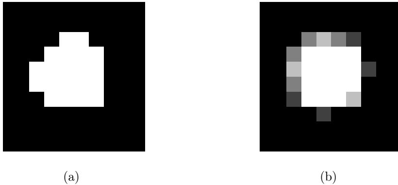
Figure 2.7: The binary and pixel coverage digitization of a disk.
