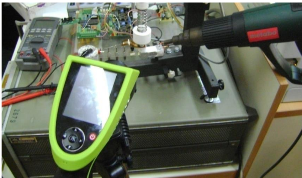
Figure 4.8 - Measurement setup for the measurement of sensor's resistance as a function of temperature
