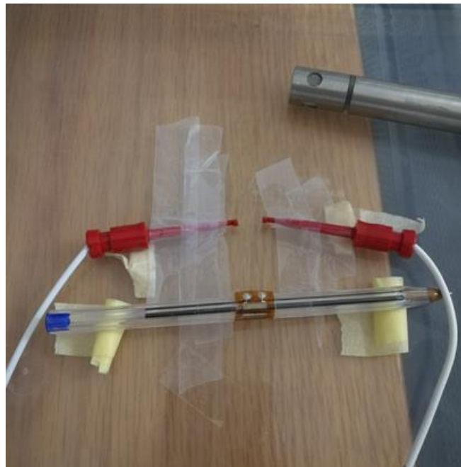
Figure 4.3 - Measurement setup used to test the flexibility influence on sensors' response.
