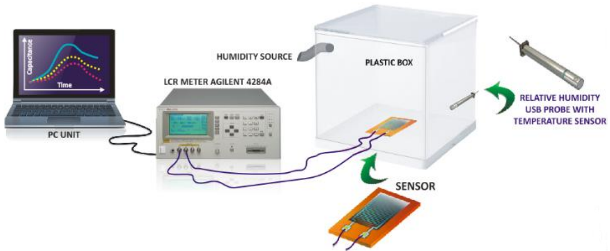
Figure 4.1 - Schematic of a humidity sensing measurement setup [20].
