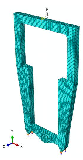
Figure 6.11 Typical FE of the frame model
