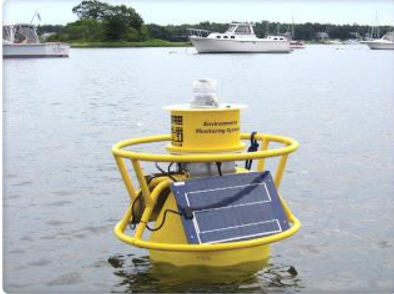
Figure 1.1. The YSI EMM68 buoy containing water quality and meteorological sensors, telemetry package, solar panels and batteries.
