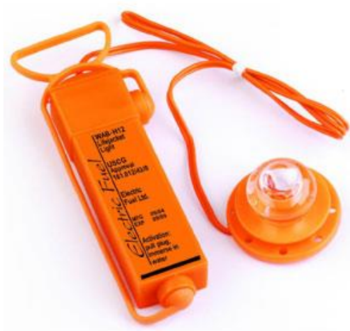
Figure 2.1. Lifejacket light, using magnesium/cuprous chloride water-activated battery ( Electric Fuel Ltd. )
