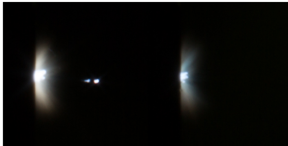
Figure 5.1: Photograph of the breakdown event with non-optimized (left) and optimized focusing (right)
