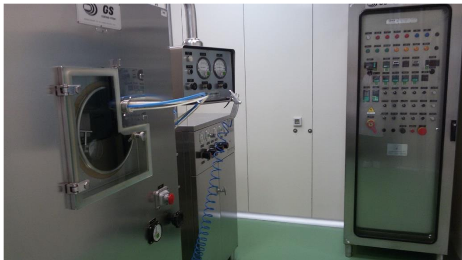
Slika 25. Uređaj za oblaganje tableta i peleta GS 25 HT/PRA/M Figure 25. Automatic coating machine for tablets and pellets GS 25 HT/PRA/M
