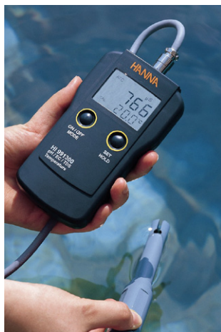
Slika 6.2.4.1 pH metar HANNA- Sigma Aldrich model C3724-1EA
