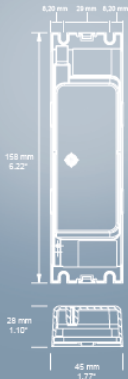
Lumen Controller NXP with Power Supply
