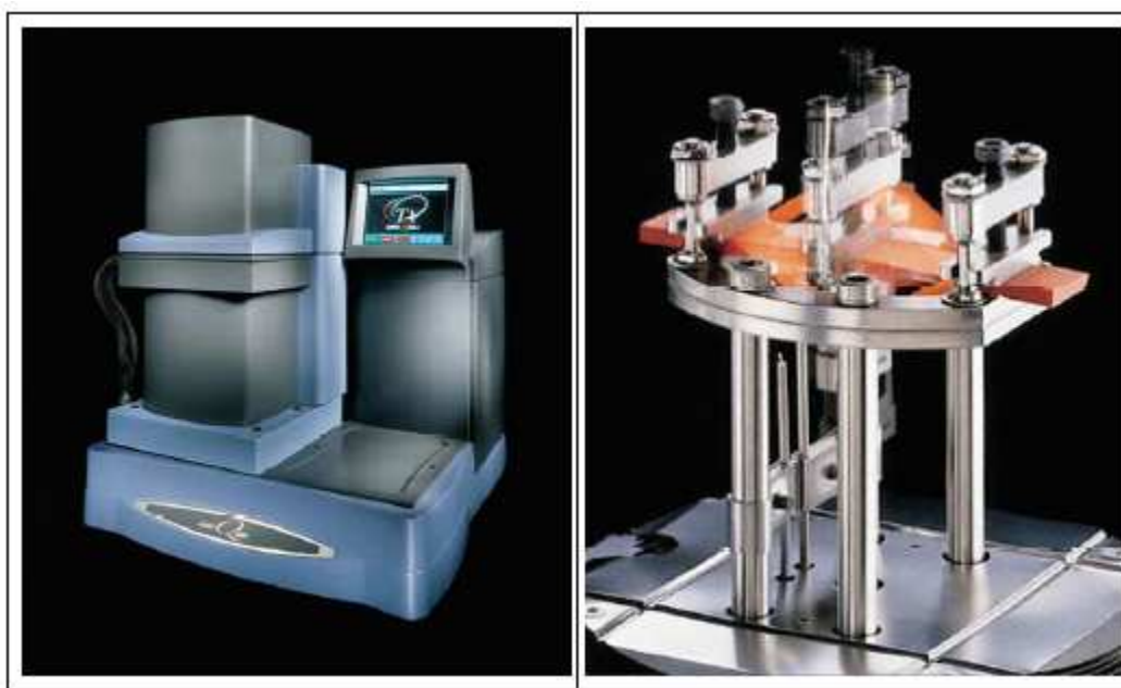
Figure 6.1 DMA Q800 (left) and single/double cantilever (right) simulating sample deformation.
